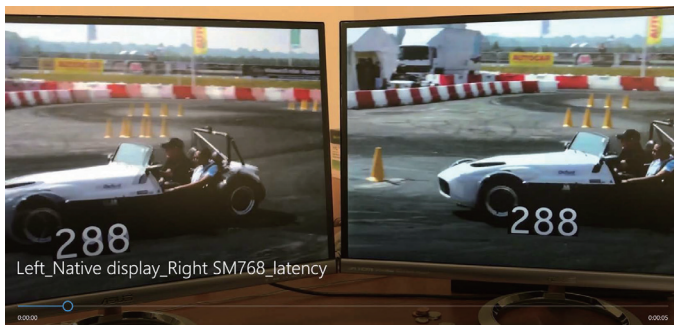
Fig.6: testing side-by-side with a native display connection shows that the latency of the SM768 is invisible
