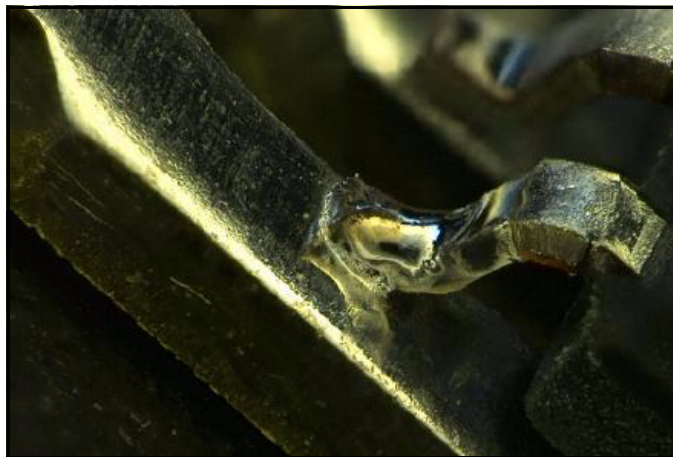
Fig. 2–7: Side view, brass leadframe
