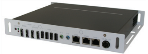
iBASE SI-28 digital signage system (10.2" W x 7.9" D x 1.4" H)
